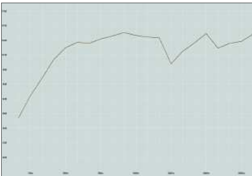
Figure 1: Axial frequency response of a multi-way loudspeaker, with the dip in response at 2 kHz due to phase cancellation between multiple drivers.
