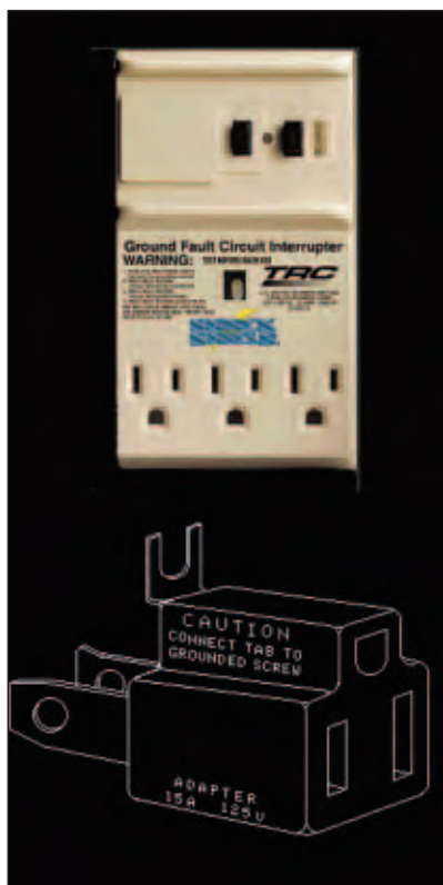
Figure 3: The GFCI (above) has a retractable ground pin that allows it to be used with a two-prong outlet. Below – it's tempting, but don't use "ground lifters" to eliminate system noise.
