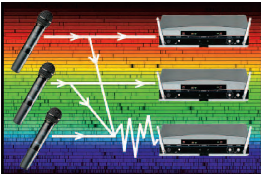
Oh no! Two systems ganging up on a third one, creating intermod – even though all three systems are on different, "clear" frequencies.
