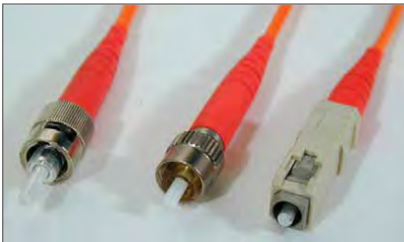
Three standard fiber connectors, left to right: ST, FC and SC.
