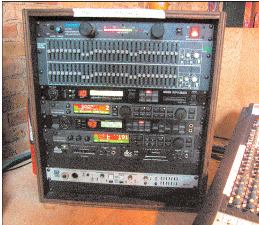
Some third-octave BSS EQ to drop in, as well as tc electronic and Yamaha effects and dbx compression/limiting.
