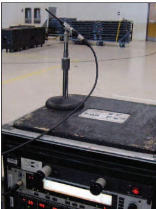
Measurement mic in position and linked via EV wireless system to SMAART.
