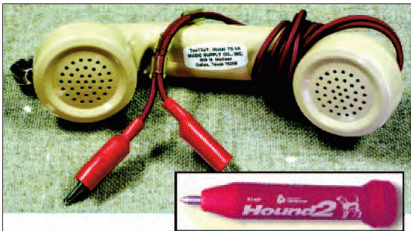
Figure 5: A passive "butt set" increases the usefulness of the ZM-104 (courtesy of www.jwdavis.com ). An inductive tester is equally useful (inset).
