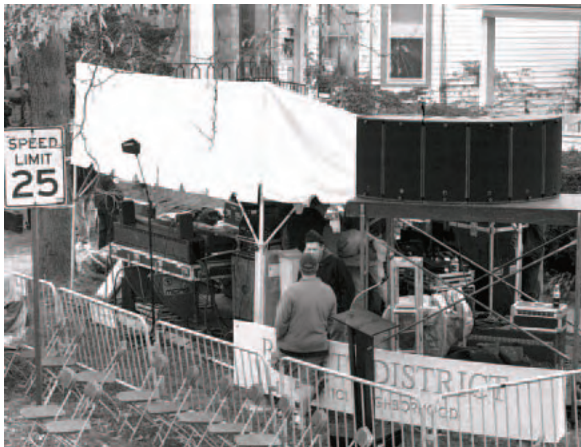
The mix position, out of the direct line of fire, flanked by L'Acoustics ARCS clusters.
