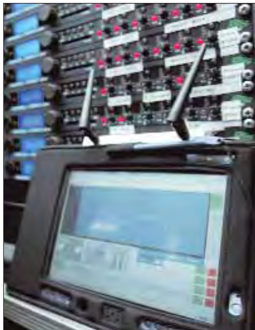
All together, the 10 Omnidrive units for Bowie's tour, and their wireless master.
